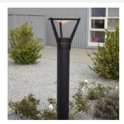
**Material & finish:** Ø30 cm top-plate with reflector in powder coated aluminium (RAL 9010, gl. 30). PC encapsulation of the light source – Ø12 cm. Black texture powder coating. Bollard Mast: Extruded aluminum
